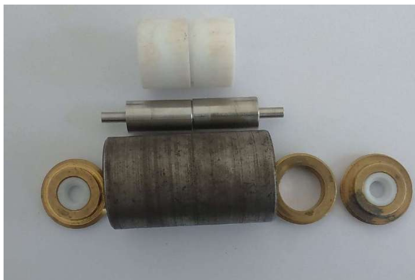
Fig. 1: Completed Newly Designed Test Cell with its Parts
